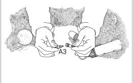
Plug in the last male plug (A3) into the female plug of the next battery pack. \*\*
